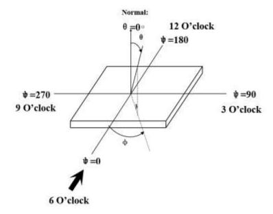
**Note 7.** Surface luminance is the LCD surface from the surface with all pixels displaying white. Refer to figure as below.
